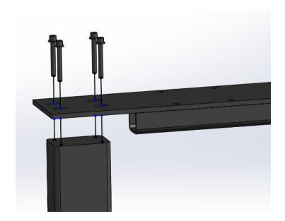
5. Attach the support bars to the upper cross piece by fastening the 5/16-18 x 3/4 Socket Head Cap Screws through the bottom of the crosspiece plates. The screws will thread into the support bar from below.
