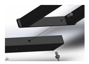
3. Fasten the upright risers to the lower cross assembly by fitting the risers into the pocketed hole in the top of each foot. Ensure the riser is seated all the way down into the foot. Fasten them together with the  $7/16-14 \times 3/4$  Hex Head Screw (Gold).
