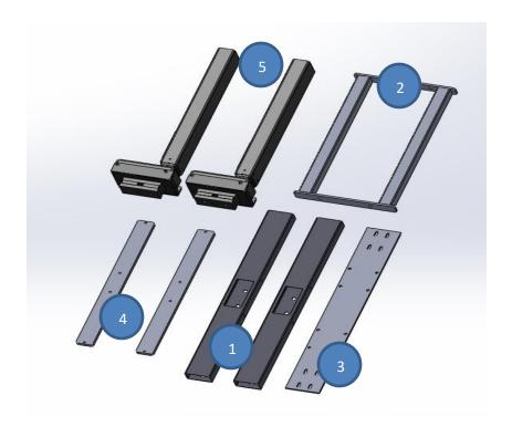
Parts 1 - 4 shown are Sound Anchors manufactured parts for the Motorized Fixed ADMID stand. Part 5 consists of Manufactured parts, along with "upright risers" and "Motor Cradle" but also consists of an electrical part from Linak. There are also other Linak components.
