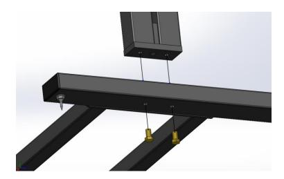
4. Attach the upper cross piece to the Top of both motors using the M6 socket head cap screws with M6 washers. There may be a need to pull the uprights together or apart from the center to ensure the crosspiece fits on the stand.
