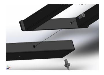
3. Fasten the upright risers to the lower cross assembly by fitting the risers into the pocketed hole in the top of each foot. Ensure the riser is seated all the way down into the foot. Fasten them together with the  $7/16-14 \times \frac{3}{4}$  Hex Head Screw (Gold).
