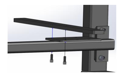
8. Attaching the 5/16-18 x 1/2 Socket Head Cap Screw to the rear hole of the support bar is optional. This screw is intended to function as a stop for speakers on our normal ADMID stands when they are tilted back. The Moto ADMID stand is not designed for tilting, but if the user chooses to adjust the spikes at the base of the stand for a slight tilt, adding these bolts to the support bar would be necessary.
