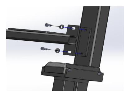
7. Attach the support bars to the upper cross piece by fastening the 5/16-18 x 3/4 Socket Head Cap Screws through the bottom of the crosspiece plates. The screws will thread into the support bar from below.
