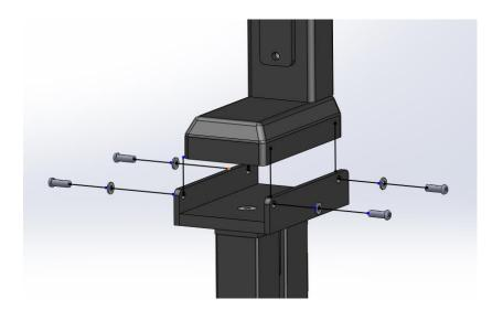
6. Attach the upper cross piece to both motors using the M8 socket head cap screws with M8 washers. There may be a need to pull the uprights together toward the center to ensure the crosspiece fits on the stand.
