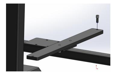
9. Lastly, tighten down any bolts left loose for fitment. Leveling should be done at this point. Add the Black & Bluedots to each end of each support bar and place your speaker on top. The Speaker should appear to be centered on the stand when you look at it from the front or the side. Keeping the center of gravity within the footprint of the stand will maximize stability and performance.
