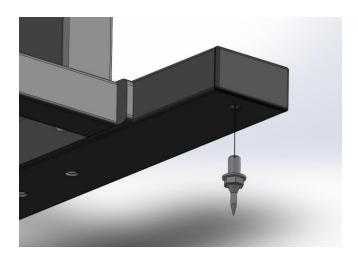
2. Fasten the 2 Feet to the lower cross piece with the 3/8-16 x 3/4 Low Head Socket Cap Screws.
