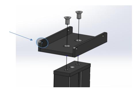
5. Attach the Motorized Lift Columns to the motor cradles by fastening them with the M6 button head screws and M6 flat washers.
